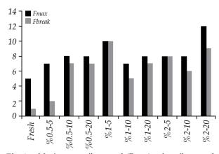
*Fig.* 4- Maximum tensile strength (Fmax) and tensile strength at break (Fbreak) of horizontal cut pericardial samples (N/mm<sup>2</sup>).
