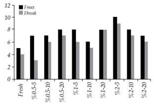
Fig. 3- Maximum tensile strength (Fmax) and tensile strength at break (Fbreak) of vertical cut pericardial samples (N/mm<sup>2</sup>)
